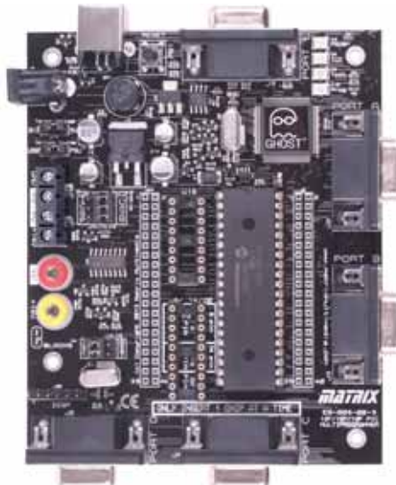
The Ghost chip on our new EB006 PICmicro Multiprogrammer enables advanced debug features.
