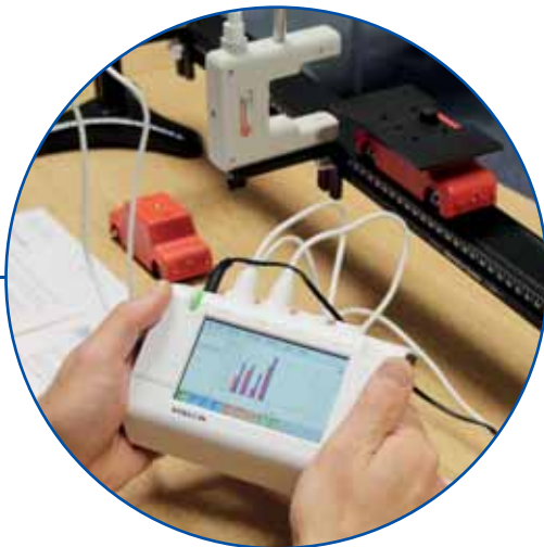
The datalogger included is fully self-contained and has a VGA output for connection to a projector for class demonstrations.
