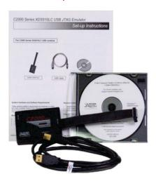
The C2000 Series USB JTAG Emulator allows the user direct access between the host computer and the TMS320C2000™ Platform DSC using the IEEE 1149.1 IEEE JTAG Interface. A JTAG emulation connection is required for debugging software, downloading code, and flash programming Texas Instruments JTAG DSCs. Compatible with Code Composer Studio IDE and supports on chip flash programming.
