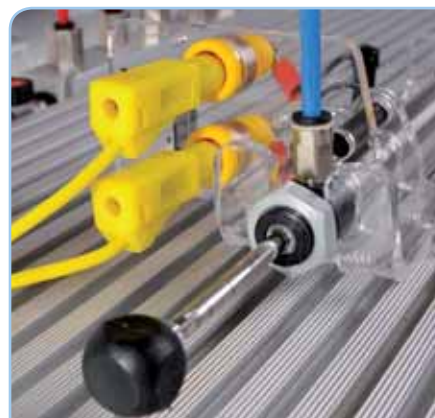
Standard 4mm cables used for all electrical connections
