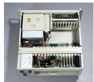
Motherboard can fit in 450 mm (17.7") depth
